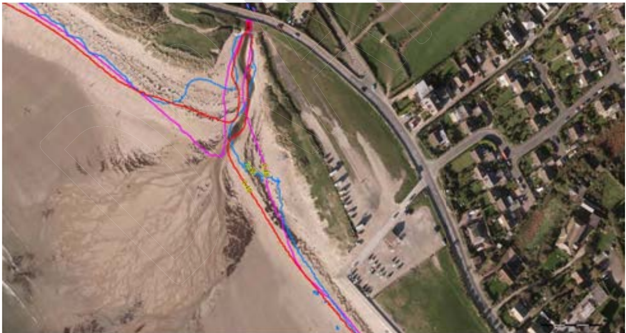
Figure 3.15 MHWs contour change at Marazion beach. Red is 2014, Blue is 2011 and Purple is 2007. Background is 2012 aerial photograph for comparison.
